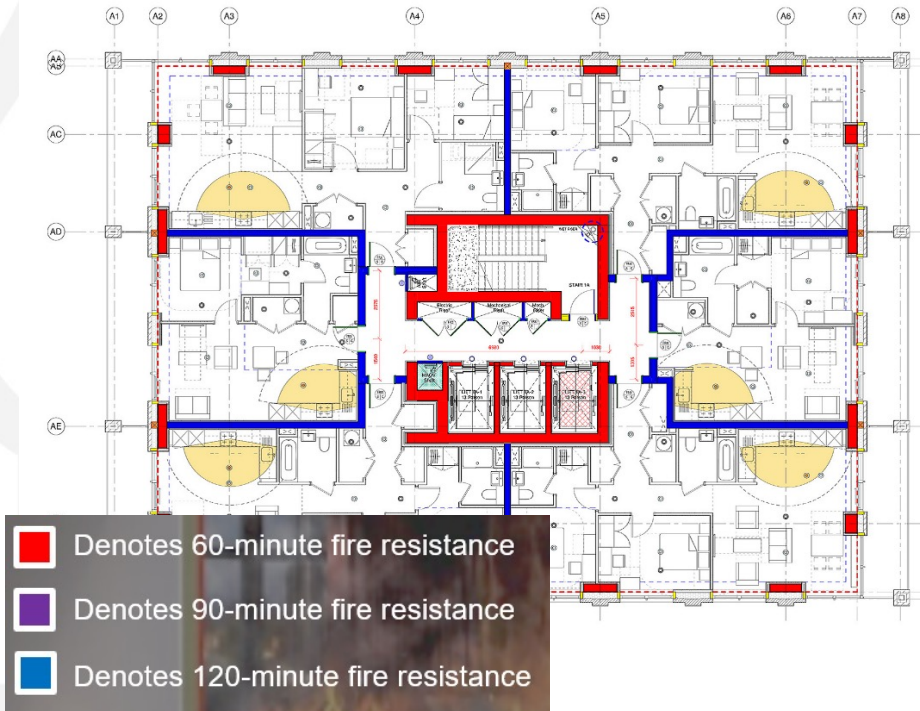
Example fire strategy drawing showing compartmentation layout
